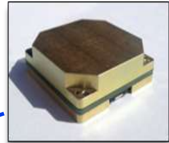
3x Tyvak Reaction Wheels - 1 mN-m torque
