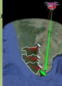
A cost effective solution is a Nano satellite equipped with a mechanism to collect data from the wireless sensor networks spread across any region
