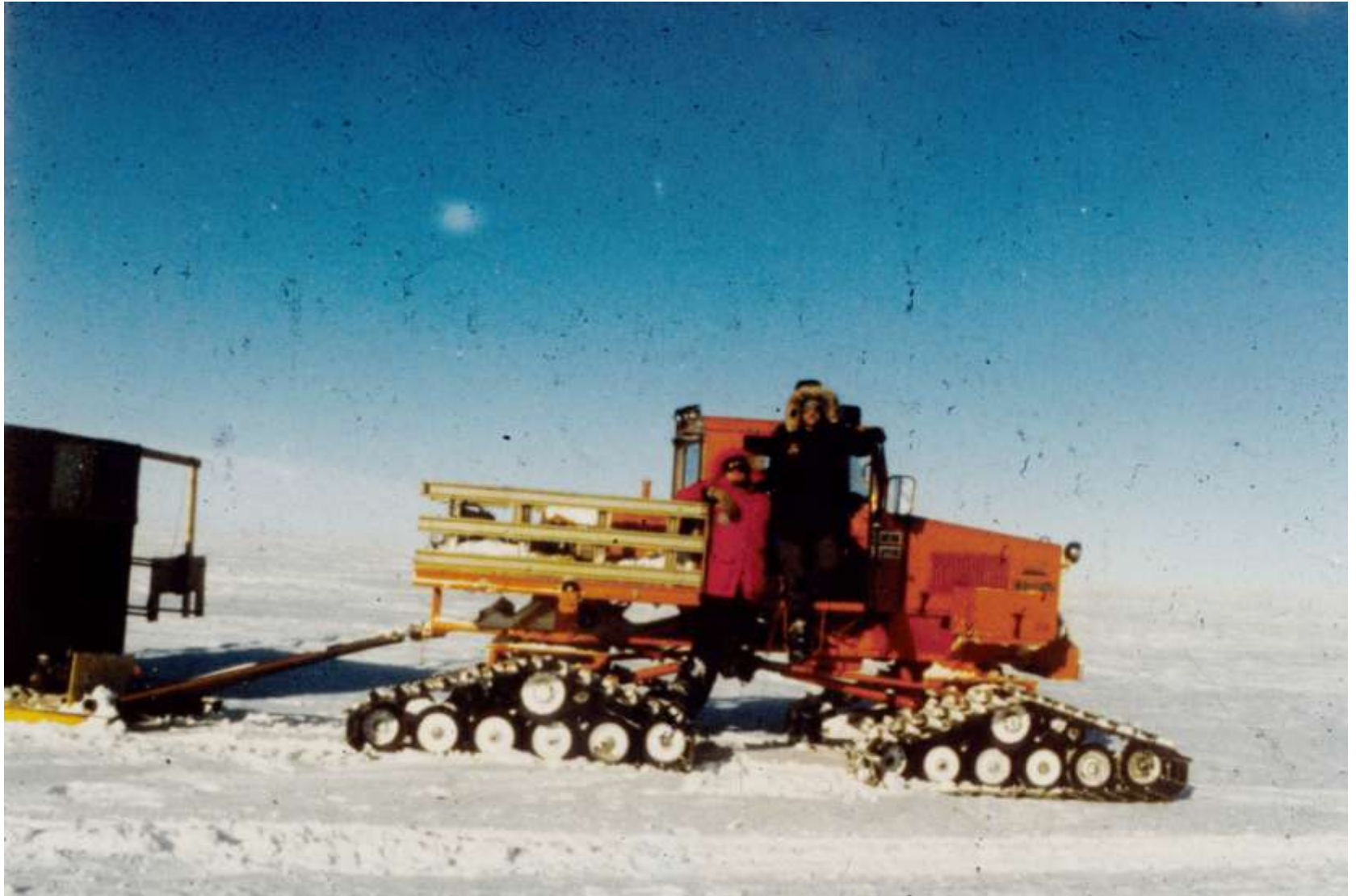
RADAR ON HUT PULLED BY A "TUCKER" ON A FAST-MOVING GLACIER – "DOWNSTREAM-B" IN ANTARCTICA
