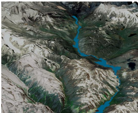
Possible flood inundation simulation in case of Sudden failure of the earthen dam (at 10000 m 3 /s) CANEUS SSTDM 2014
