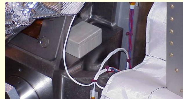
Micro-Triaxial Accelerometer Unit installed on MPLM – 2 Shuttle Missions since 12/01
