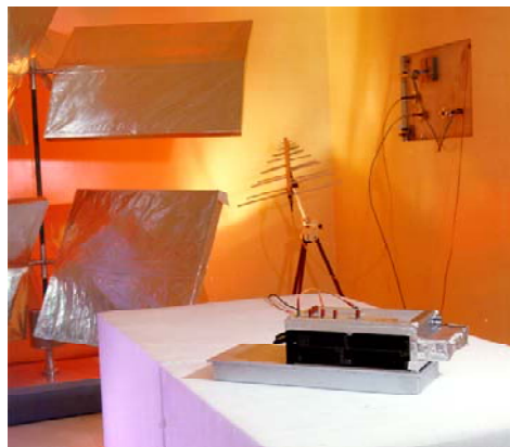
NASA/Honeywell RCS in HIRF Chamber
