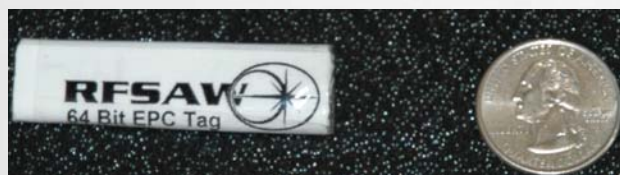
64-bit SAW-based COTS RFID tag
